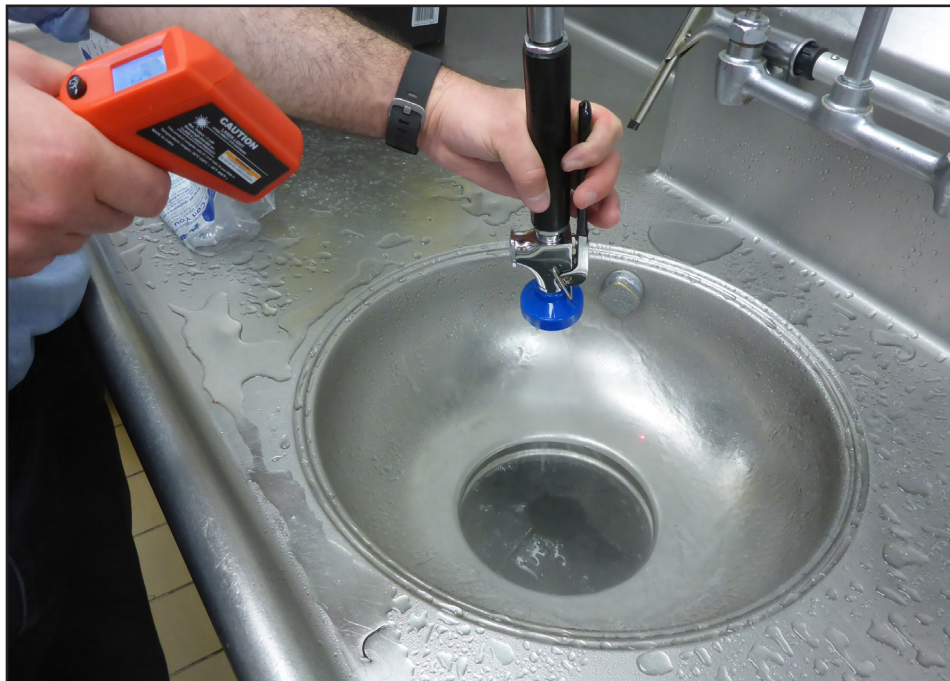
A retrofit pre-rinse spray valve undergoes a water temperature test to ensure that it meets the needs of the facility for proper operation. Retrofitting older pre-rinse spray valves with newer efficient models can help reduce water and energy bills on military installations. (Photo by Elisabeth Jenicek)
